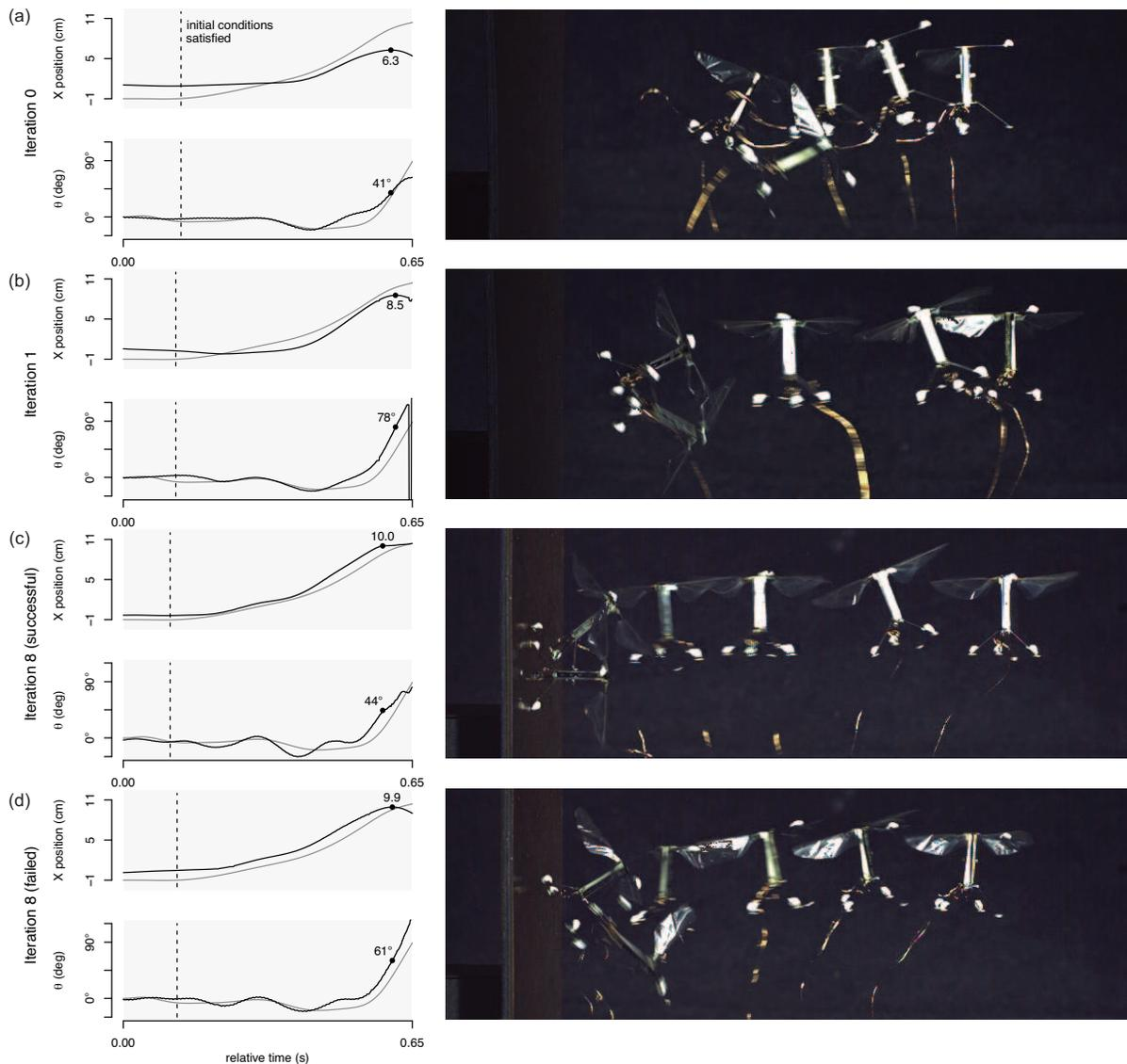
Fig. 6. Recorded trajectories accompanied by composite images constructed from the videos. References are shown in grey lines and the actual trajectories are in black lines. (a) The trajectory obtained without any command from the ILC algorithm. (b) The trajectory generated after one learning iteration. (c) A successful trajectory obtained after 8 iterations of learning. (d) A failed perching attempt obtained from the same command as in (c).
