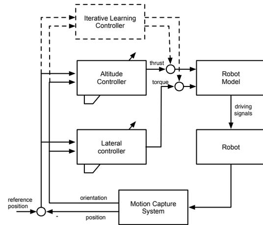
Fig. 3. A block diagram illustrating the feedback control architecture of the robot. The ILC control block (in dashed lines) is implemented in addition to the existing closed-loop system.
