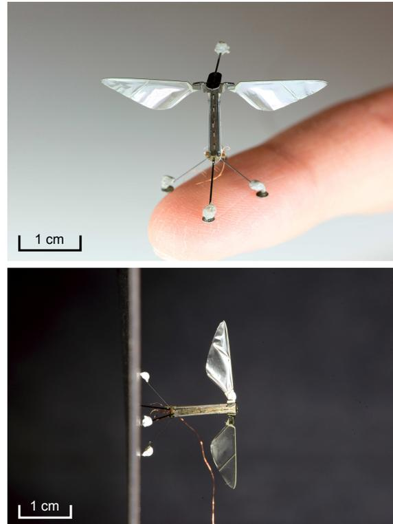
Fig. 1. (top) Photograph of a biologically-inspired robotic fly on a finger with four retro-reflective markers for tracking purposes.. (bottom) A robot attached to a magnetic wall via the aid of 6mil steel shims attached to the base of the landing gear.
