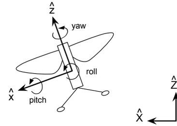
Fig. 2. Definitions of the inertial frame, the body-attached frame, and roll, pitch, and yaw axes.
