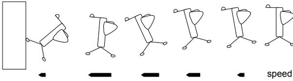
Fig. 4. A schematic diagram demonstrating how the robot can perch on a vertical wall. Initially it needs to build up sufficient forward momentum to retain it when the robot rotates to the opposite direction at the moment of landing on the wall.
