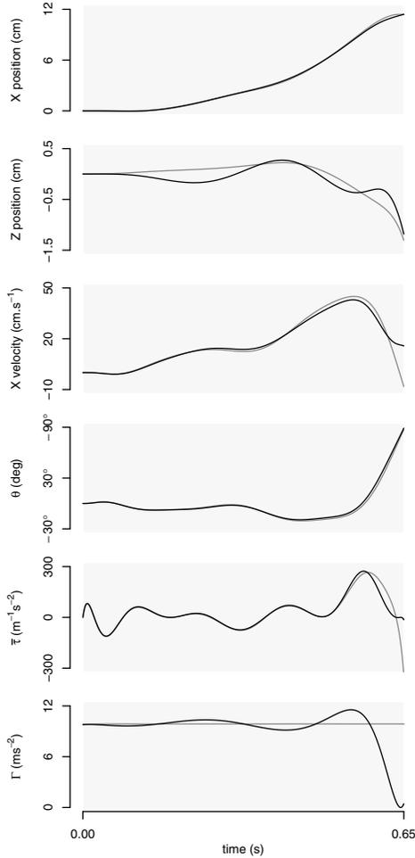
Fig. 5. A candidate trajectory for perching. The grey lines show a parametrized version of a hand-designed trajectory. Black lines represent the final trajectory after the optimization.
